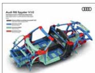
Figure 1. Example of application of different materials in the construction of a car structure [4]
